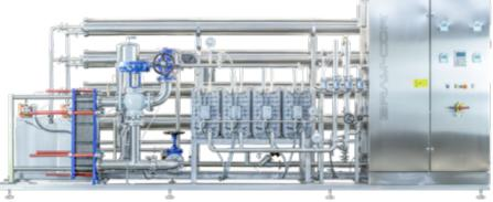
**CROS Reverse Osmosis Systems** are designed to produce compendial Purified Water (PW), Ultrapure water and/or "cold" Water for Injection (WFI) through several water treatment steps, depending on feed water quality and production needs. Water treatment steps, which are necessary to separate the water from organic substances, high and medium molecular weight ions and from some bacteria and pyrogenes, can include:
