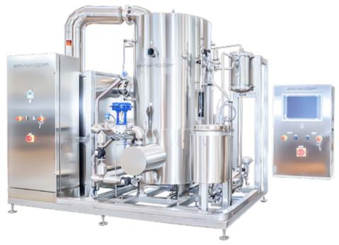
BRAM-COR **STMC Vapor Compression Distillers** produce compendial Water for Injection for pharmaceutical applications, such as I.V. solutions, injectables, washing systems and special solutions where both quality factors (sterility, elimination of pyrogens and of chlorine solvents with low molecular weight), and economical factors, as well as the low production costs, are critical for the success of the pharmaceutical process.
