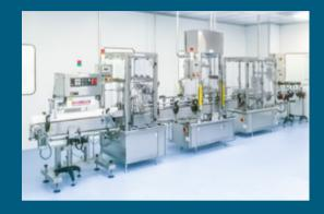
BRAM-COR pharmaceutical bags or bottles filling machines are intended for automatic, semiautomatic or manual use, for different bags or plastic/glass bottle sizes, depending on production requirements (from min. 50 ml). In addition to ensuring trouble-free operation, our equipment reduces maintenance costs and ensures long-term reliability. Complete bottle lines are integrated with washing machines, capping and crimping machines, labelling lines and belt conveyors. Our Filling & Packaging lines:
