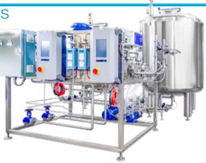
stantly monitored by ozone analyzers, while residual ozone in water is automatically removed by a sanitary UV lamp before PW use in the process. Sanitary piping, valves, pumps and instruments complete each **GENO** unit.
