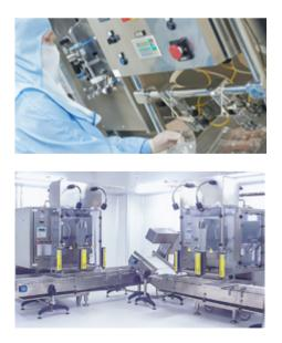
The capping process of the **BFIL S** and **BFIL A** models is automatic and eliminates the need to manually insert plugs into the filling pipe. The feeding of the plugs can be both manual or automatic, through vibrators, the capacity of which depends on the kind of plug used.
